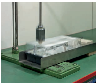
In impact tests according to DIN EN 50102, the maximum mechanical stress of the materials is tested using spring hammers and drop hammers.
